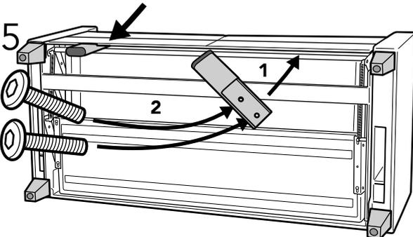
Mount the support leg in place and screw the 2 (M6X25mm) bolts into the pre-drilled holes.
