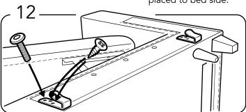
Mount the 2 anchors with M6x20mm bolts and 15mm screws as shown in pictures. Use the bolt in upper hole and 2 screws on other holes. Do not overtight the screws!
