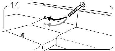
Put down the bed headside part and attach the bed backside to the chaise backside with 2 (M6x50mm) bolts.
