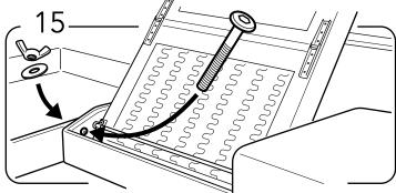
Lift up the bed mechanism part and attach the bed at front with butterfly bolt set.
