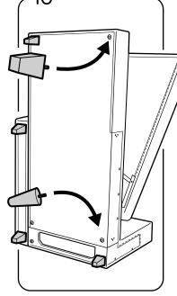
Attach the legs to the openable chaise The additional leg allways placed to bed side.
