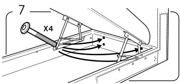
Now lift up the openable chaise part and attach the backside with 4 (M6x50mm) bolts
