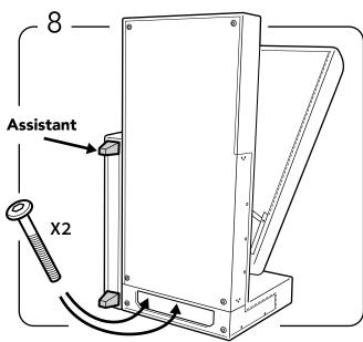
Turn the openable chaise to backside and let the assistant hold the armrest as shown in picture. Fix the armrest to the back from inside the frame with 2 previously removed bolts.
