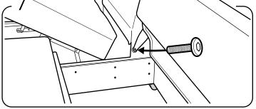
Attach the backrest to the chaise part (don't forget to use the two washers between).
