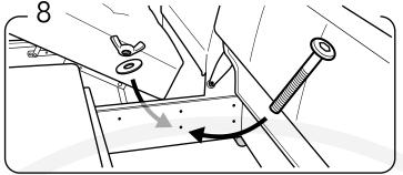
Mount the bed to openable chaise by using one bolt set on backside.
