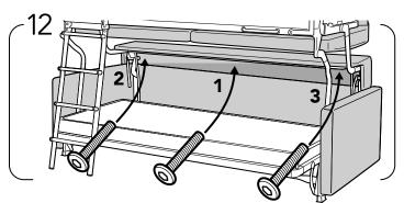
Use the M6 x 30mm bolts as shown on picture 11. After tightening the frst bolt in the middle. Tighten the bolts to the edges.
