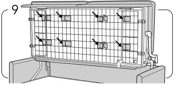
Open the bed mechanism as shown on picture and leave it to first resting position. Tighten the right and footboard and headboard. Tighten structure to the lift seats . Slip the fixing blades between the bottom parts of upper bed.
