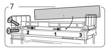
Attach the front panel. Use the M6 x 20mm bolts Tighten first bolt in the middle and edges after that.
