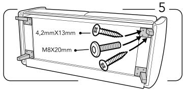
Attach each legs with the M8x25mm bolt to align the metal in place then use two screws on each leg.
