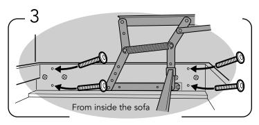
Fasten sofa frame to left and right armrest with a 4 (M6 50 mm) bolts in each side.
