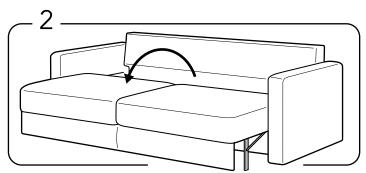
Place lift and right armrest in place, and open the mechanism completely.
