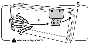
Mount the metal leg in place and screw the 4 (3,5mmX25mm) woodscrews.
