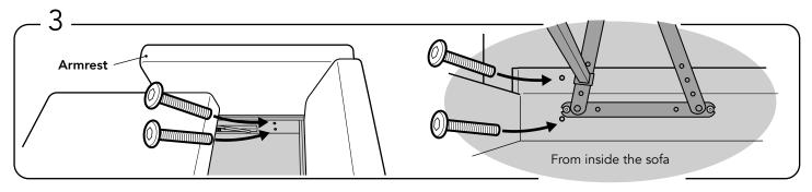
Fasten sofa frame to left and right armrest with a 4 (M6 50 mm) bolts in each side. All bolts fastened from inside out!
