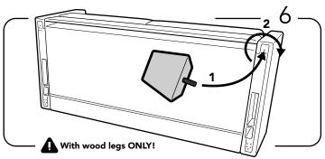
Mount them in place by twisting each clock-wise into the pre-drilled holes.
