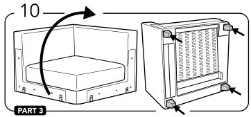
Turn the corner to the backside, Then insert the 4 legs.
