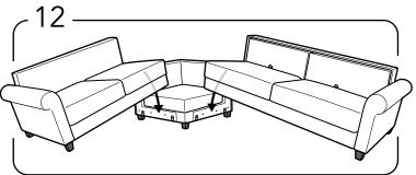
Attache the bed and the stationery parts to the corner part inside the pre-installed anchors.
