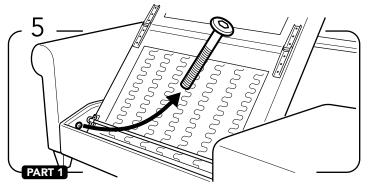
Remove the frontside armrest fixating bolt.
