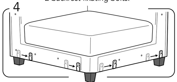
Re-position all the anchors as shown in the image above in the pre-drilled holes.
