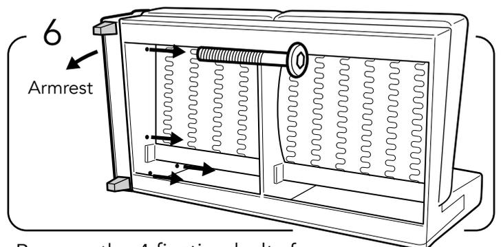
Remove the 4 fixing bolts from inside the stationery.
