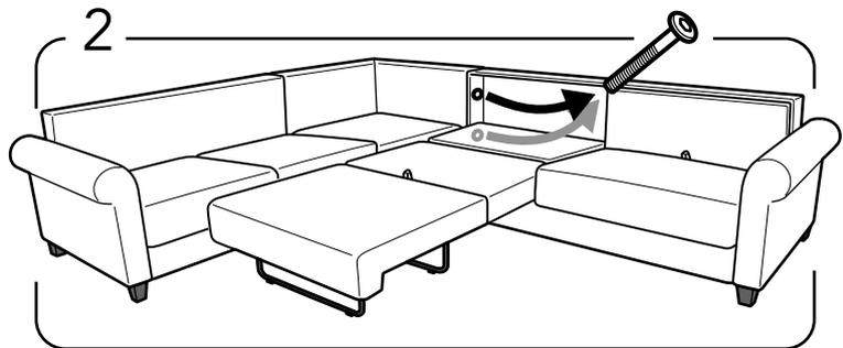
Open the bed mechanism, then remove 2 backrest fixing bolts.
