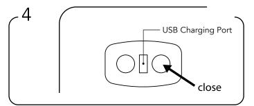
To close the sleeper, press and hold the close button. An audible beep will sound when the deepest seat position is reached. To continue, release and press again until closed fully.
