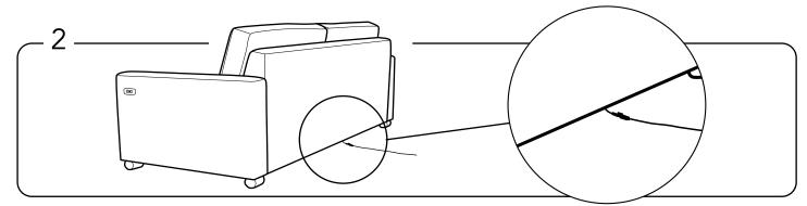
Connect the power cord to in the back of the sleeper. Plug the power into an outlet.
