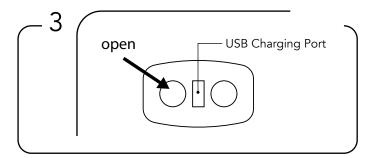
To operate press and hold the open button. An audible beep will sound at the deepest seat position, release and re-press until the sleeper opens fully, and the motors stop.
