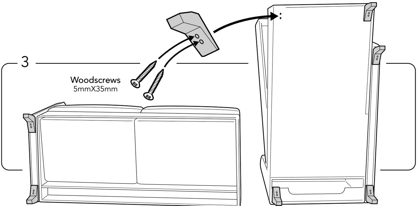
Attach each legs with the 2 (5mmX35mm) Woodscrews in the pre-drilled holes.
