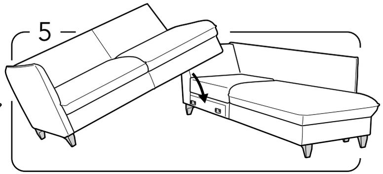
Attach the loveseat with the chaise part as shown on picture. Be sure that the both metal brackets are attached correctly!
